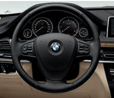
■ Leather steering wheel with multifunction buttons for operating the Cruise Control and the radio or telephone.
