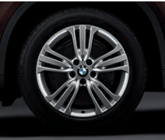
□ 19" light alloy wheels W-spoke style 447 with mixed tyres, front 9 J x 19 with 255/50 R 19 tyres, rear 10 J x 19 with 285/45 R 19 tyres.
