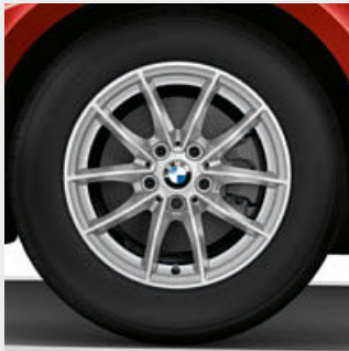
■ 16" light alloy wheels V-spoke style 774 Reflex Silver, wheel size 6.5J x 16, with 205/60 R16 tyres. 1
