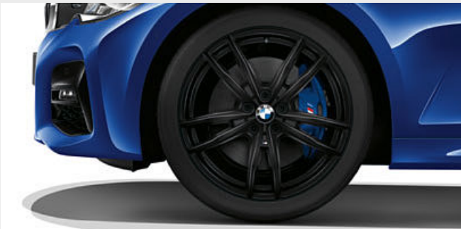
□ 19" M light alloy wheels Double-spoke style 791 M Jet Black uni with mixed tyres and runflat tyres, gloss-lathed, front 8J x 19 with 225/40 R19 tyres, rear 8.5J x 19 with 255/35 R19 tyres. 6
