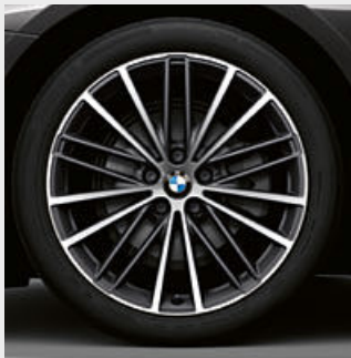
□ 19" light alloy wheels V-spoke style 635 Ferric Grey gloss-lathed with mixed tyres and runflat tyres, front 8J x 19 with 245/40 R19 tyres, rear 9J x 19 with 275/35 R19 tyres.
