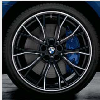
○ 20" M Performance light alloy wheels, forged, in Bicolor Black matt, milled and gloss-lathed on the visible side. Complete wheel set with run-flat tyres.
